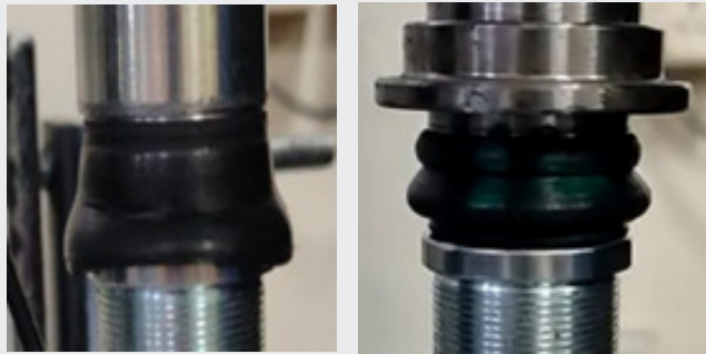
Fig. 4. Compressed behaviour of Initial (Left) and new (Right) design bump stop
